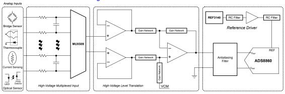
OPA4991-EP in a High-Voltage Signal Chain
