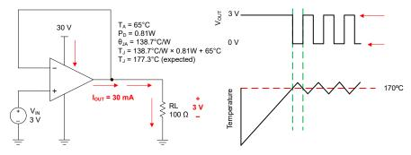
Figure 7-4. Thermal Protection
