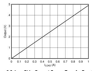
Figure 8-2. Low-Side, Current-Sense, Transfer Function
