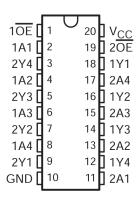
Figure 3-1. DW or PW Package, 20-Pin SOIC or TSSOP (Top View)
