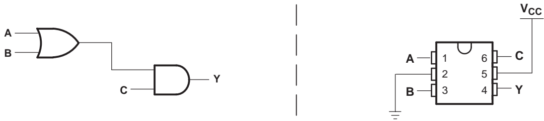
Figure 3. Y = (A + B) \bullet C
