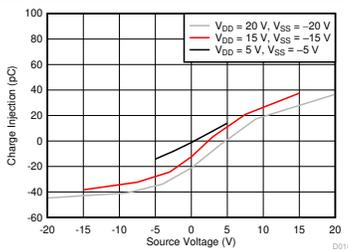
Figure 5-15. Charge Injection vs Source Voltage – Dual Supply
