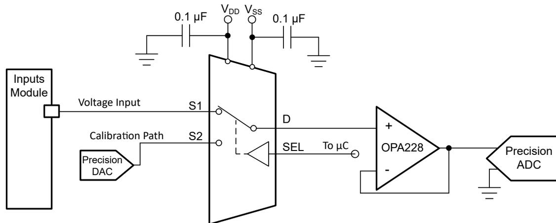
Figure 8-1. Calibration Path Switching for Data Acquisition
