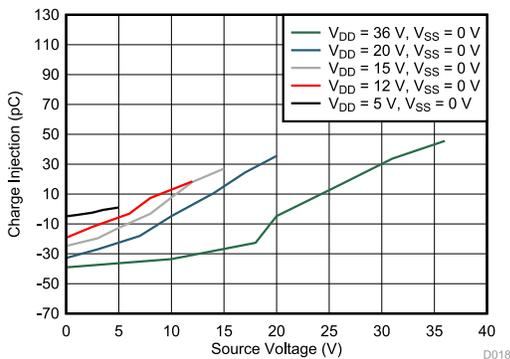
Figure 5-17. Charge Injection vs Source Voltage – Single Supply
