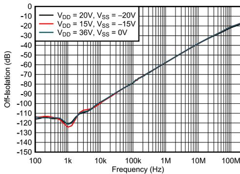
**Figure 5-23. Off-Isolation vs Frequency**
