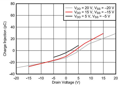
Figure 5-16. Charge Injection vs Drain Voltage – Dual Supply
