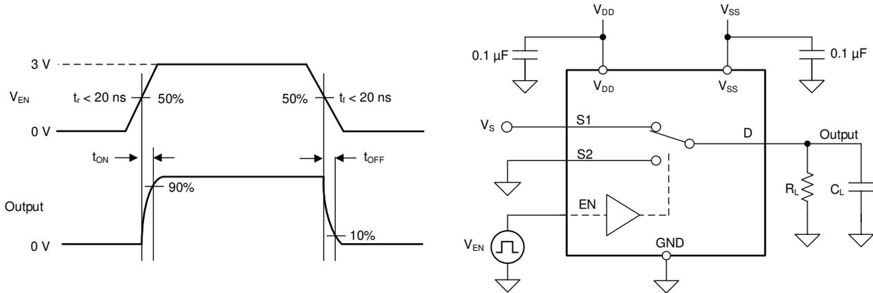
Figure 6-5. Turn-On and Turn-Off Time Measurement Setup
