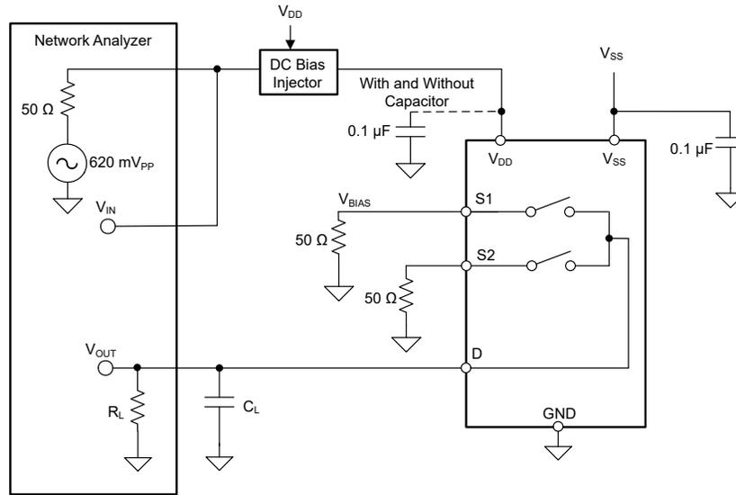
$$\text{PSRR} = 20 \times \text{Log} \frac{V_{\text{OUT}}}{V_{\text{IN}}}$$
