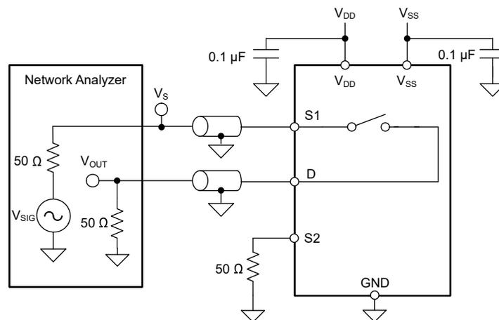
$$\text{Off Isolation} = 20 \times \text{Log} \frac{V_{\text{OUT}}}{V_s}$$
