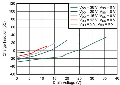
Figure 5-18. Charge Injection vs Drain Voltage – Single Supply
