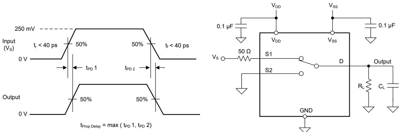
**Figure 6-8. Propagation Delay Measurement Setup**
