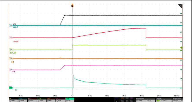
Figure 8-7. Power Up Into Short: V_{IN} = 54V , EN/UVLO Stepped Up From 0V to 3V
