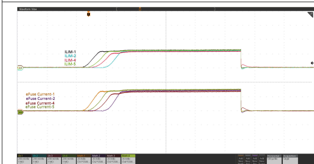
Figure 9-8. Power Up into Short (Current distribution among five devices in parallel): V_{IN} = 12 V, EN/UVLO Stepped Up From 0 V to 3 V, R_{IREF} = 40.2 k \Omega , R_{ILIM} on Each Device = 300 \Omega , and OUT Shorted to GND
