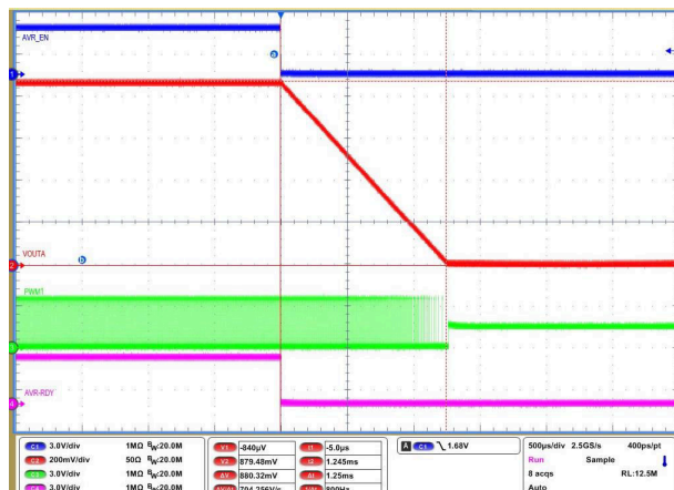
Figure 8-9. Soft-stop channel A (0 ms TOFF_DELAY)
