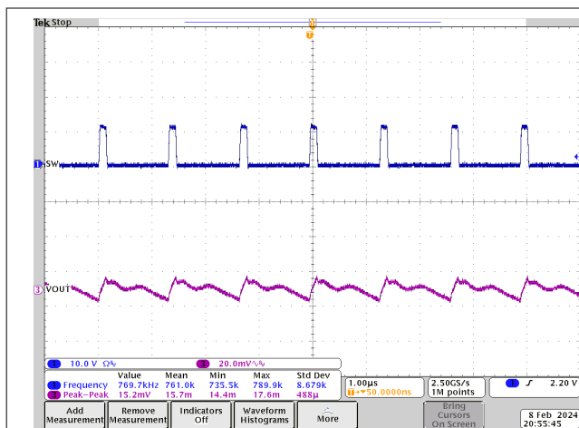
Figure 7-14. Output Voltage Ripple, 800kHz FCCM, 40A Load, PVIN = 12V, VOUT = 1.1V
