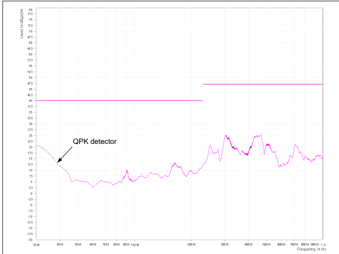
Figure 9-8. CISPR 32 Class B Radiated Emissions: Horizontal Polarization
