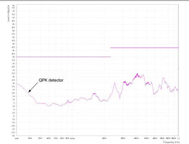
Figure 9-9. CISPR 32 Class B Radiated Emissions: Vertical Polarization
