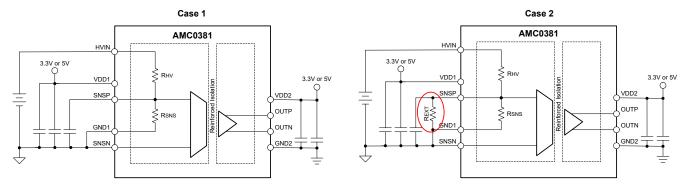
Figure 2-7. Gain Error Resistor Divider Variation Schematics
