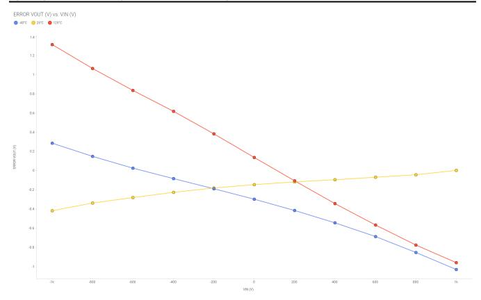
Figure 2-5. Total Output Referred Error Voltage vs. Input Voltage
