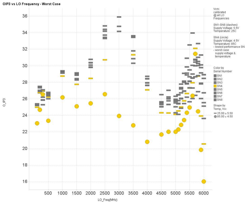
Figure 13. TRF370417 OIP3 vs LO Frequency – All Frequency Calibration Comparing 4.5 V at 85°C to 5.5 V at 25°C
