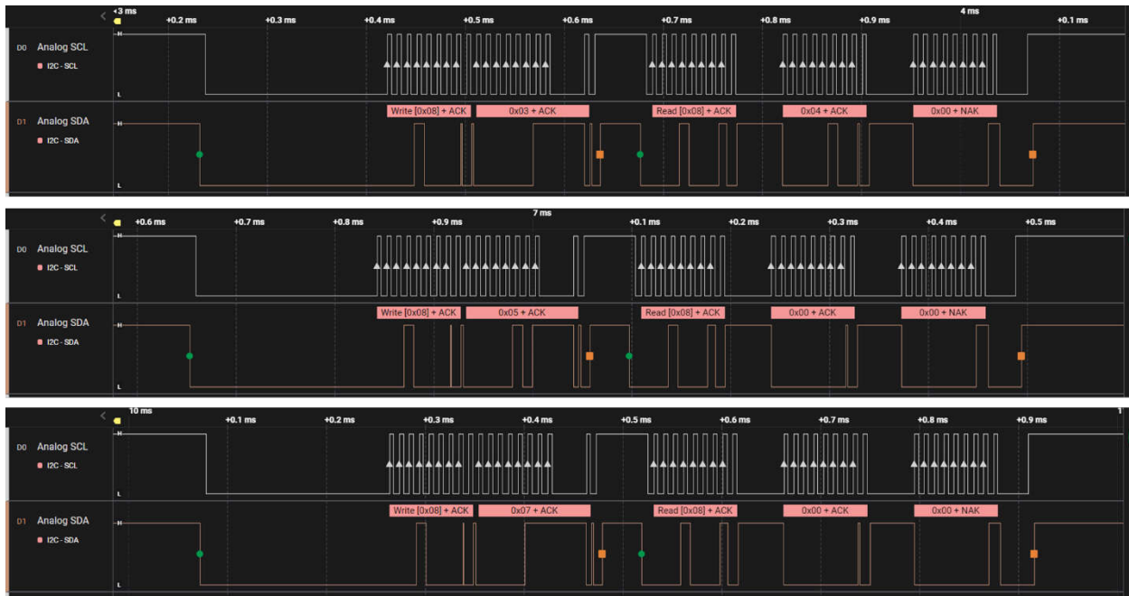
Figure 4-2. Captured I2C Waveform for Safety Status Reading
