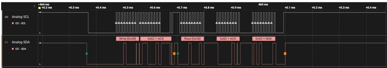
Figure 4-1. Captured I2C Waveform for Alarm Status Reading
