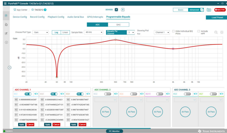
Figure 3-4. PurePath™ Console Programmable Biquad Filter Example Showing the Computed Coefficients in Normalized Floating Point Format
