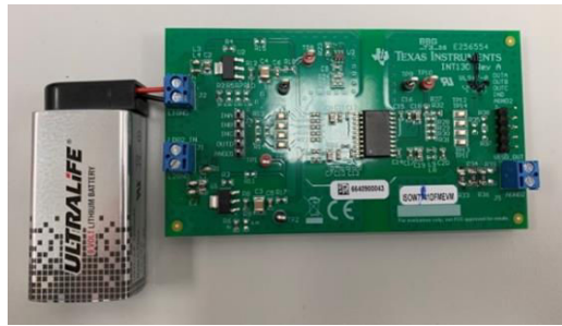
Figure 7. ISOW7741 evaluation module
