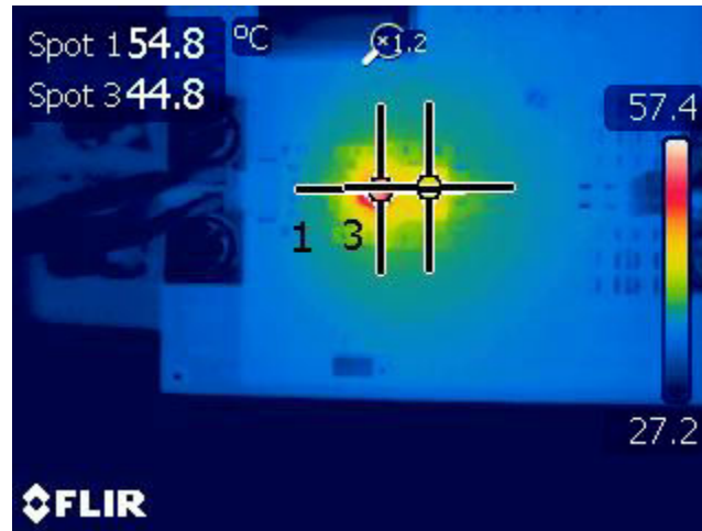
Figure 3. Single TPS6287B25 Supplying 0.45V Rail at 20A DC With 3.3V V_{IN} at Room Temperature
