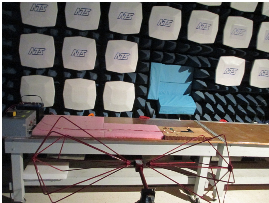
Figure 3. Setup for Radiated Emission (RE) – Bi-con Antenna Horizontal for 30 MHz to 200 MHz Range
