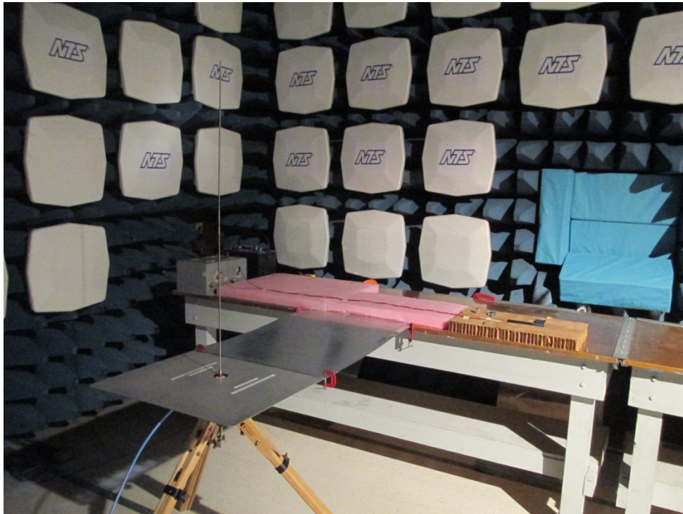
Figure 2. Setup for Radiated Emission (RE) – Monopole Antenna (Rod) for 150 kHz to 30 MHz Range
