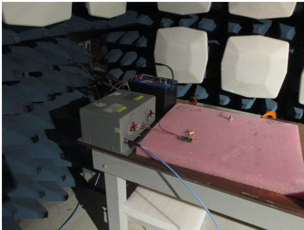
Figure 1. Setup for Conducted Emission (CE) Measurements
