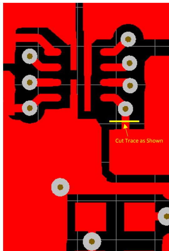
Figure 1. Loop Response Measurement Modification
