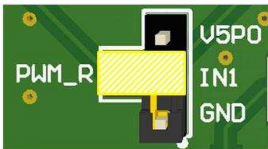
Figure 5. IN1 Connected to PWM Output
