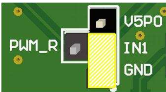
Figure 3. IN1 Connected to GND (Logic Low)
