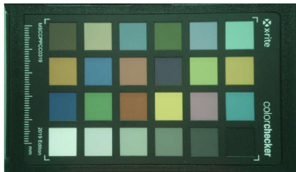
Figure 7-6. Image After Black Level Subtraction
