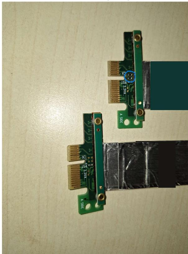
**Figure 4-1. Modified PCIE\_FLEX\_CLK cable**
