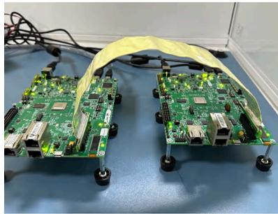
**Figure 4-2. Two AM64x Connected Though Unmodified PCIe Cable**
