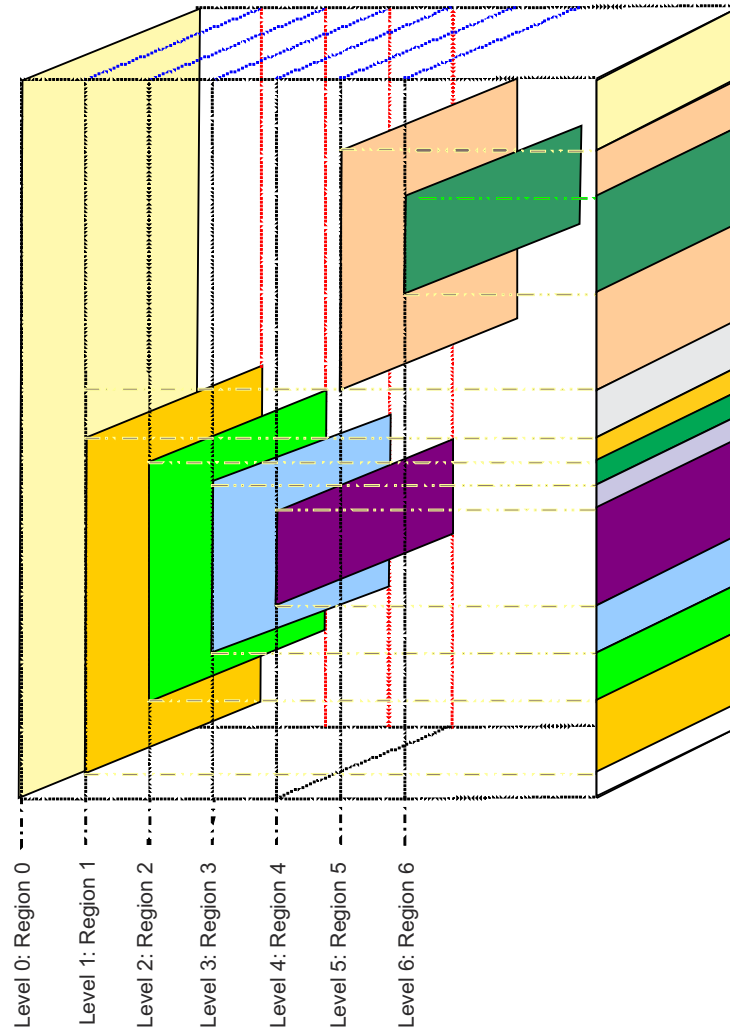
Figure 14-6. L3 Interconnect Region Overlay and Priority Level Overview
