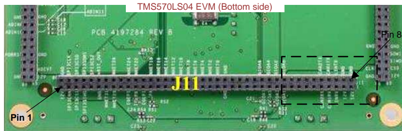
Figure 3-19. Safety MCU EVM Interface
