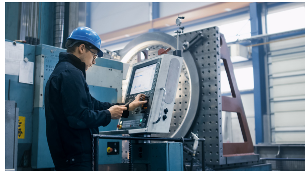
Figure 6: CNC machine with large HMI
