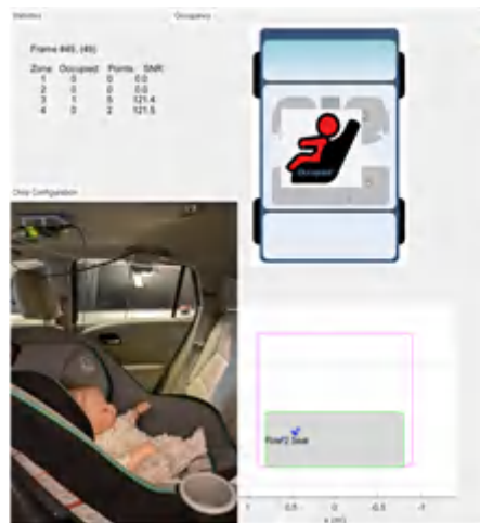
Figure 1. (a) Detection of a child (Baby Doll) in the front driver footwell, (b) front passenger seat rear-facing, and (c) 2 nd row driver-side rear-facing inside SUV using the AWRL6432.
