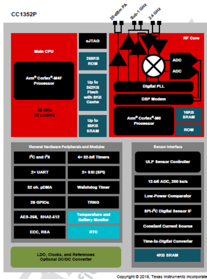
Figure 3. SimpleLink CC1352P Block Diagram
