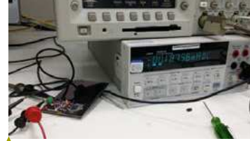
Figure 15. 250 LUX Light Intensity Measurement Setup
