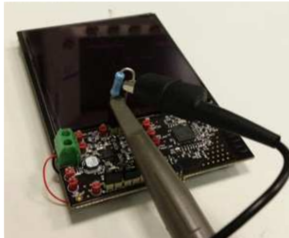
Figure 12. Current Probe Measurement for Dynamic Power Measurement
