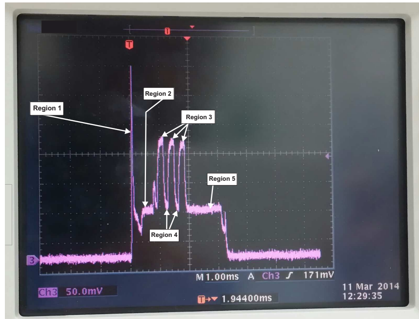
Figure 13. Power Drawn During Beacon Transmission
