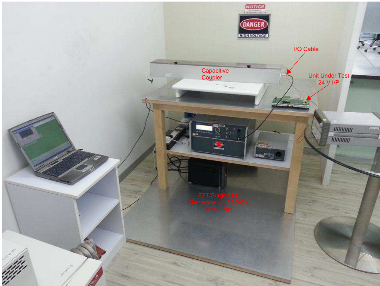
Figure 35. Pre-Compliance Test Setup
