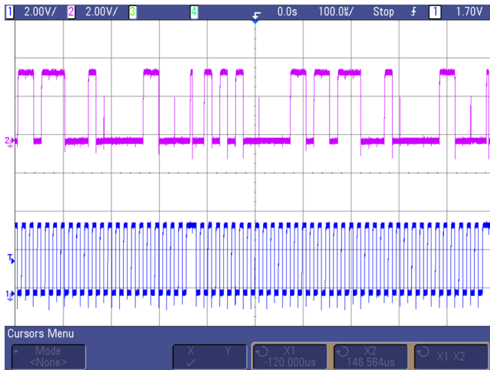
Figure 15. I 2 C Communication Showing SDA Signal (Pink) and SCL Signal (Blue)
