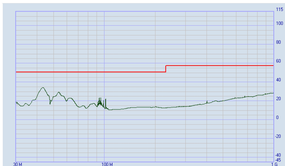
Figure 22. DC/DC 24-V Buck HotRod™ Package Radiated Emission J1
