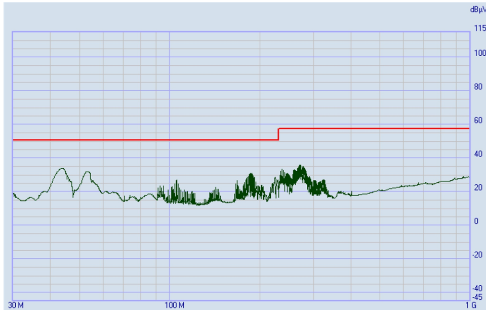
Figure 21. DC/DC 12-V 5-V Buck Power Module Radiated Emission
