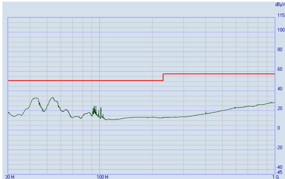
Figure 19. DC/DC Buck Power Module Radiated Emission J3
