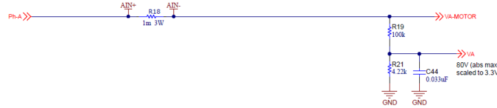
Figure 3-4. Phase A Voltage Sense Circuit
